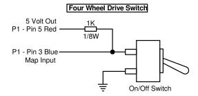
For this setup you need to put the switch on in the software on the negative edge.
