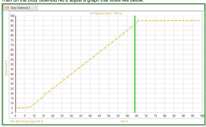
At Low duty cycle the solenoid will be on and front wheel drive will work. As the pedal is pressed deeper then mode drive will be transferred to the back wheels engaging 4x4. At maximum duty cycle the four-wheel drive lock will be fully engaged.
