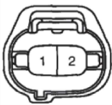
NB! Harness Plug Pin View
