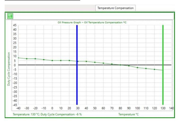
This graph is used to compensate line pressure with temperature. A cold transmission will shift harder. Depending on specific firmware this graph will compensate either line pressure or shift control pressure. The example above is line pressure. If it is for shift pressure the graph may have a rising slope.
