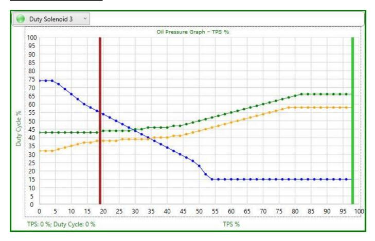
This graph will determine the line pressure which acts on the clutches. This pressure is a pulse width modulation signal and is calculated according to the throttle position. It is critical that the TPS is calibrated and operates correctly.
