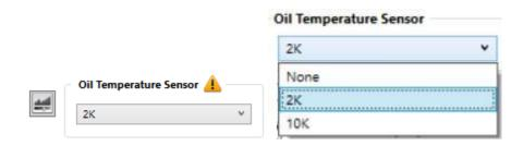
This signal is a critical setting which means it is saved separate from the 4 maps. It can only be calibrated in MAP 1 and does not change when other maps are loaded in the TCU. The Clone function will alter this calibration to the Clone map.
