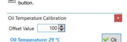
Now adjust the offset value to match your accurate thermometer. Click the *OK* button. Then click on the *Save to TCU* button to make the changes permanent.
