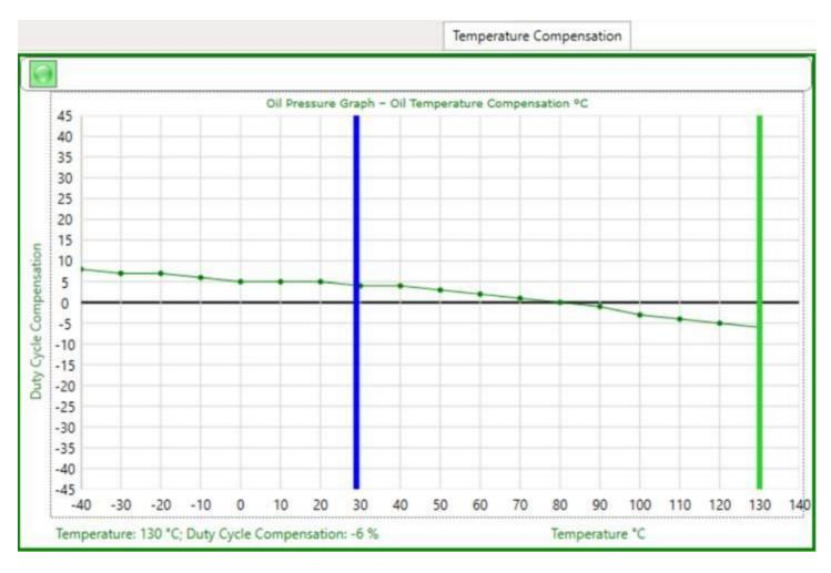
This graph is used to compensate line pressure with temperature. A cold transmission will shift harder. Depending on specific firmware this graph will compensate either line pressure or shift control pressure. The example above is line pressure. If it is for shift pressure the graph may have a rising slope.
