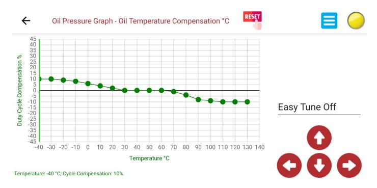
This graph is used to compensate line pressure with temperature. A cold transmission will shift harder. Depending on specific firmware this graph will compensate either line pressure or shift control pressure. The example above is line pressure. If it is for shift pressure the graph may have a rising slope. See the Specific Instructions for each transmission.
