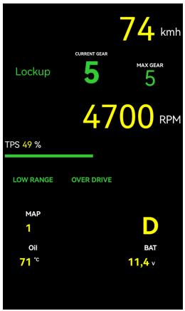
This block displays all the analogue sensor values as they change in the ECU. Below is a description of the meaning of each signal.
