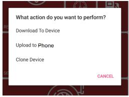
Download to Device means the map will be loaded in the ECU but the Critical Settings will not be changed.
