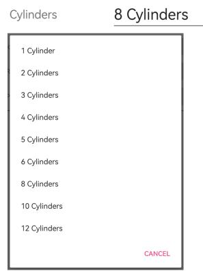
Number of cylinders on the engine can be selected in this block. It is not used by the current firmware but reserved for future development of different firmware.
