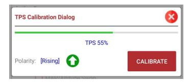
The TPS value must increase with throttle depression. If it is decreasing, click on *Polarity* to select *Negative*. This feature is normally used where the original ECU is still connected and wiring cannot be altered. In this case you connect only the ECU TPS signal wire to the OEM signal wire. Do not connect the ground or 5-volt signal wires but isolate them to prevent shorts. Now click the *Calibrate* button. The current TPS value will be written into the two blocks *Min* and *Max*.
