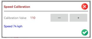
Change the offset value till the speed value reads the same as the car speedometer, or as a GPS
