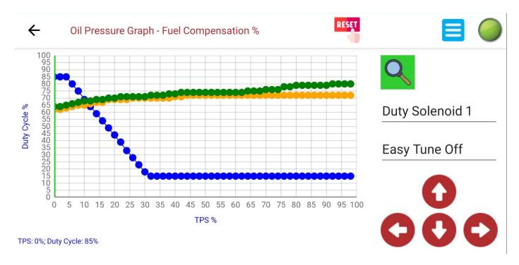
This graph will determine the line pressure which acts on the clutches. This pressure is a pulse width modulation signal and is calculated according to the throttle position.
