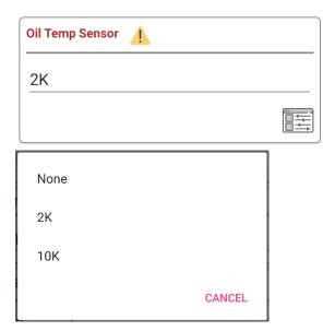
This sensor indicates transmission oil temperature to the TCU. It is not used in all TCU firmware but it does help to smooth shifting when the transmission is cold. There are 2 selections for different sensors. Normally 2k or 10k which alter the sensor calibration. Note that this does use a different wire in the harness as well. Select None if it is not used.
