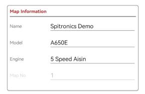
The Map information screen, **Name Model** and **Engine**, contains info for the TCU application for a specific vehicle. This helps the tuner to recognize previous work and tuning data. It is saved in the TCU and also in PC maps. It does not affect any tuning on the engine.
