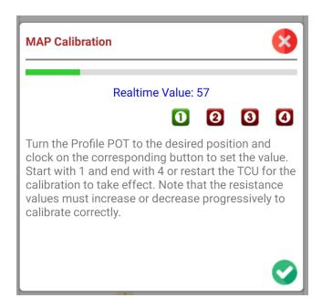
Put the Map switch in position 1. As a test you can go through all the positions to position 4 to see if the real time value change significantly.
