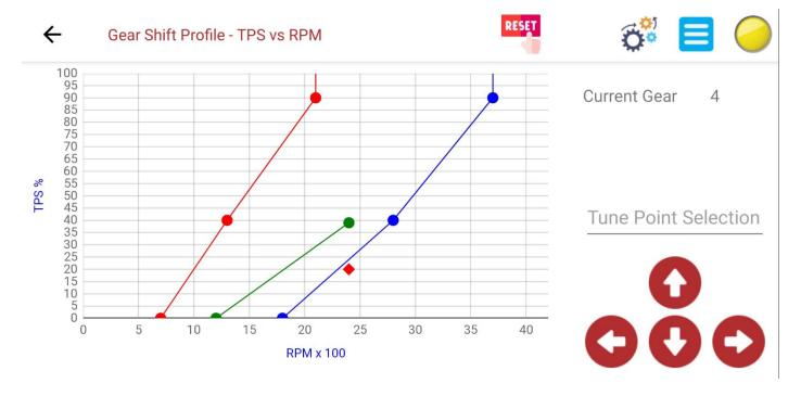
These profiles are used to set up each gear to shift on its own pattern and according to certain criteria. This feature will let the installer set up the TCU for custom drive trains to the desire of his customer. The up and down shift algorithms can be manipulated with ease.
