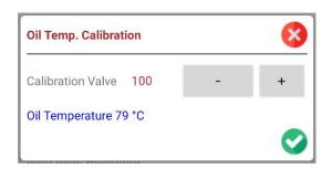
Now adjust the offset value to match your accurate thermometer. Click the *OK* button. Then click on the *Save to TCU* button to make the changes permanent.
