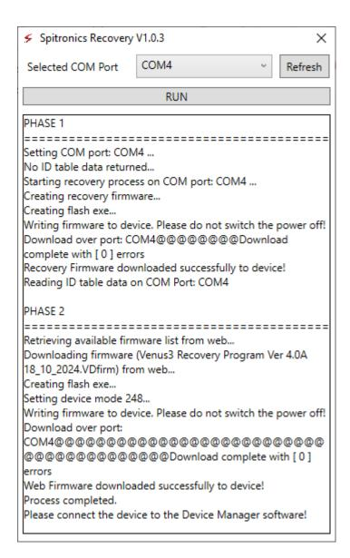
You can now close the recovery software and open **HS DM4**. From there, proceed to load the correct firmware for the Venus3. Once you loaded firmware connect with HS ECU software and go through your setup again and make sure your map file is still ok and no settings have changed. Once you are sure your ECU is setup correctly you may switch the device off and connect the other connectors.
