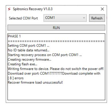
If the incorrect Comm Port is selected, the message will look like this: "???" in the string, indicating no response from the device. However, if the correct port is chosen, you'll see "@@@" in the message, confirming the communication was successful. See the picture below. The Firmware select block will now open, allowing you to load the X\_Test Firmware version 4.0. This will enable you to open Hyperspace Device Manager 4.0, from which you can install the correct firmware.
