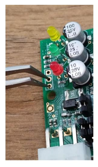
Once the jumper is in place, switch the power on. The **Green1 LED** will light up. Now, remove the jumper from the communication connector. The **Green1 LED** will turn off, indicating that the Venus3 is now in Program mode.
