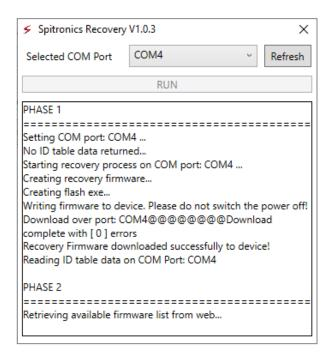
Select the **Venus3 Recovery Program Ver 4.0A 18\_10\_2024.VDfirm** and click **OK**. If the message shows "@@@" again, the programming was successful. This firmware will not pulse any outputs so it is safe to use in a car. Only the 4 LED's on the mercury will flash indicating the firmware loaded successfully.
