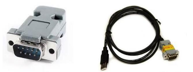
The Prolific RS232 to USB converters were popular in the old days and could be used only for TCU, EMU and Titan units. Note however that you had to break-out pins 1, 4, 6, 7, 8 & 9. This is due to other connections from the ECU to the 9 pin D-sub connector. Use a small screwdriver and bend them outwards and then inwards till they break out. Do not damage the other pins. There are small numbers inside. Below is an illustration of the layout.
