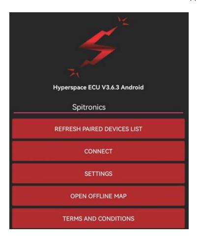
If connection cannot be made click on Settings and make the Poll Error Count 3 or more till the connection is stable and the green LED pulse stable.
