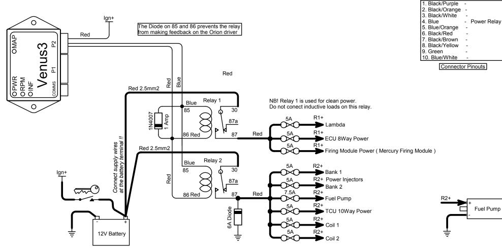
**NB!** Relay 2 is used for inductive loads. If you have more than 3 Coils use a third Relay to share the load. Try and keep Coils on their own relay. Add the 6 Amp Diode on to pin 87. It will prevent inductive spikes from the coils to damage lower voltage drivers of the injectors.
