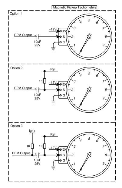
**Note:** The connection to the ECU changes with the GP Output Priority selection. View the Priority spreadsheet for the specific firmware to see which output is selected. Then make sure on how to connect between the 2 options above. It could be connected on a negative or positive driver.
