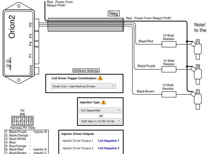
Injector Driver Output 3 Coil Negative 3
