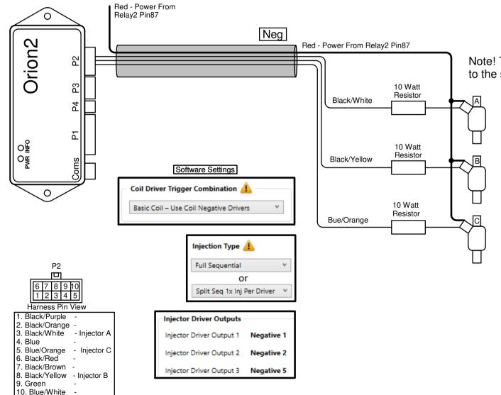
Note! The 10 Watt resistor must be close to the same value resistance as the injector
