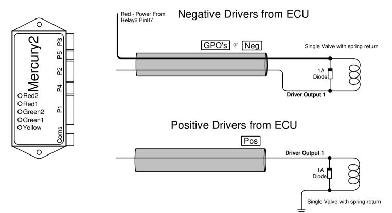
**Note:** The connection to the Mercury ECU changes with the GP Output Priority selection, View the Priority spreadsheet for the specific firmware to see which output is selected. Then make sure on how to connect between the 2 options above. It could be connected on a negative or positive driver.
