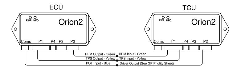
**Note:** The connection from the Orion2 TCU changes with its GP Output Priority selection. View the Priority spreadsheet for the specific firmware to see which output is used as Retard output. It will be a negative driver.
