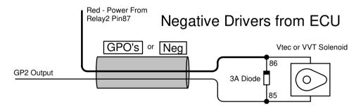
**NB!!** The Diode must be connected. Make sure the stripe on the diode is facing the positive.
