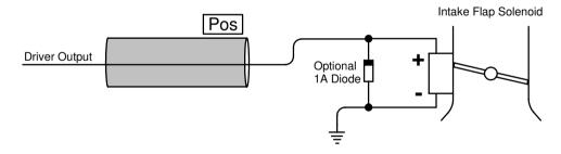
**NB!!** The Diode must be connected. Make sure the stripe on the diode is facing the positive.
