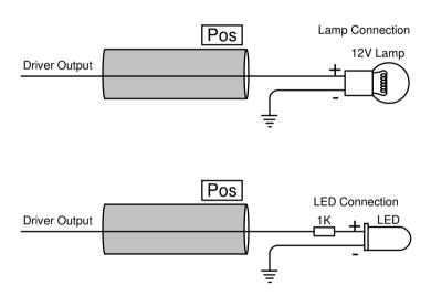
**Note:** The connection to the ECU changes with the GP Output Priority selection. View the Priority spreadsheet for the specific firmware to see which output is selected. Then make sure on how to connect between the 2 options above. It could be connected on a negative or positive driver.
