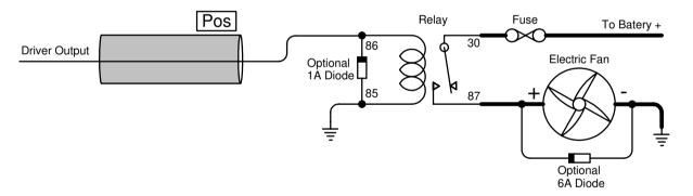
**Note:** The connection to the ECU changes with the GP Output Priority selection. View the Priority spreadsheet for the specific firmware to see which output is selected. Then make sure on how to connect between the 2 options above. It could be connected on a negative or positive driver.
