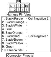
Coil Driver Trigger Combination
