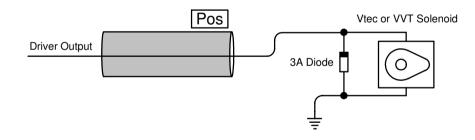
**Note:** The connection to the ECU changes with the GP Output Priority selection. View the Priority spreadsheet for the specific firmware to see which output is selected. Then make sure on how to connect between the 2 options above. It could be connected on a negative or positive driver.
