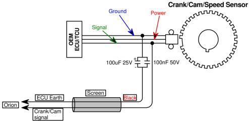
Note: See drawing for corect wire color of the specific sensor.
