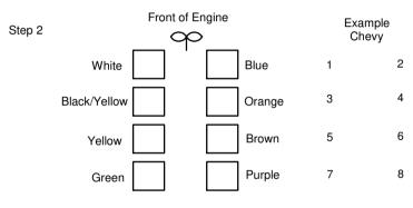
Write the cylinder layout of your engine in the blocks above. Make sure which side is the No1 cylinder and how they are numbered on your engine. Then write the corresponding colour of each cylinder next to your coil number on the lines marked X on the drawing. This will ensure that the sequence of spark is correct.
