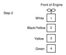
Write the cylinder layout of your engine in the blocks above. Start with No1 cylinder in the front and fill it in to the back. Note that it will not be numbered as the cylinders but acording to the fire order. Then write the corresponding colour of each cylinder next to your coil number on the lines marked X on the drawing. This will ensure that the sequence of spark is correct.
