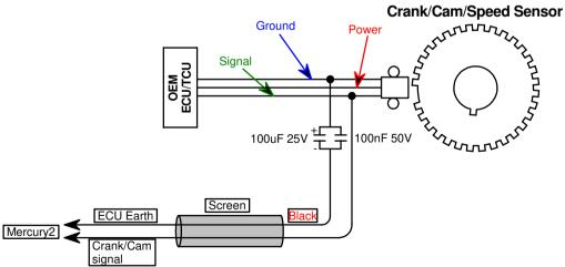
Note: See drawing for corect wire color of the specific sensor.
