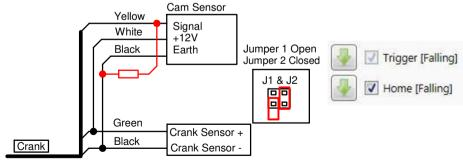
Note! Optional 1 K resistor from signal to earth will help prevent interference from the ECU supply voltage
