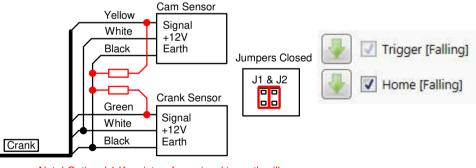
Note! Optional 1 K resistors from signal to earth will help prevent interference from the ECU supply voltage
