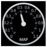
This value displays the manifold pressure and is scaled according to the MAP range setting.
