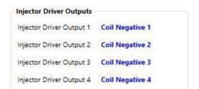
On Hyperspace 3.6 Software the Injector drivers are now also displayed. This will indicate how many drivers are allocated to Injectors and will change according to Injector Type setting. This will allow the installer to do a printout of the drivers after setting up his unit.
