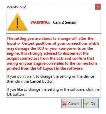
All Critical settings will be saved separately in the Orion2 which means when you load a map they will not be changed. Except if you press the Clone button. Critical settings can only be altered on a live device or with the clone function.
