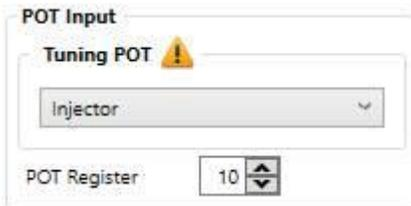
**Injector** setting will change the injector time with 10% richer or leaner in this example. The POT needs to be in the middle to have no effect on current fueling. This is handy in a race car if the driver has an A/F Ratio gauge installed. Then he can manipulate fueling and remember under which conditions he has to lean or richen the mix. Then he can make adjustments on the graph at a later stage.
