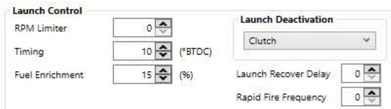
Now connect the relevant wires from the TCU to the ECU. When the TCU makes a shift it will put a negative driver on. It will connect to the POT input of the ECU. The POT real-time bar will be high and the moment of shift it will go low, activating the retard feature.
