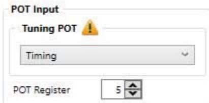
**Timing** will advance or retard the ignition timing by 5 degrees in this example. The POT needs to be in the middle to have no effect on current timing. It is useful in racing for tuning time while driving. Ensure that the driver has a knock sensor and light fitted to the engine.
