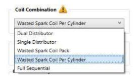
This block indicates the type of coil combinations that can be used with this firmware. Some firmware programs will allow the user to select between the different coil combinations on his engine. **Note**: If you have an intermediate or lower hardware class ECU, you may only use single coil with distributor. Most COP coil per cylinder engines are fired in wasted spark configuration and each coil will have its own driver. (See the wiring diagrams for connections.)
