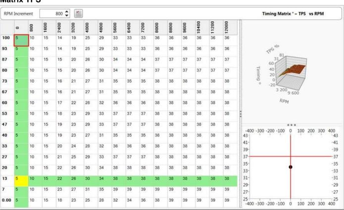
This is for normal aspirated engines with poor vacuum signal or throttle bodies and allows for easy dyno tuning. Note: It is recommended to add the altitude sensor to compensate for altitude pressure changes. TPS versus RPM does not compensate for pressure changes. Here the TPS sensor versus RPM is used and the blocks are set in 1-degree resolution.
