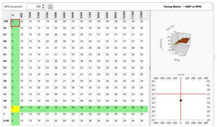
This is for standard engines with a good vacuum signal and allows for easy dyno tuning. Here the MAP sensor versus RPM is used and the blocks are set in 1-degree resolution.
