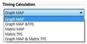
This block will allow the tuner to choose different options to set up timing for this engine. Each of these methods will be discussed in detail under the tuning chapter further in the manual. You can see the *Tuning* section for detailed description on the tuning side.
