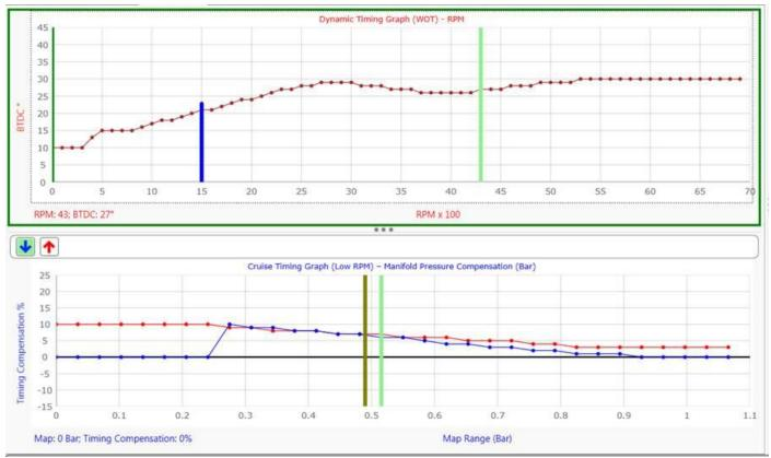
This method is for standard engines with a good vacuum signal and it allows for easy tuning in the street. It has a Dynamic timing map on top which is tuned at WOT. It has 2 vacuum tuning maps for pull-off and cruise timing adjustments.
