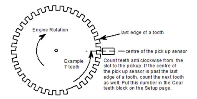
With the engine running match the timing as close as possible by using the Gear teeth setting. For example; the ECU software indicates 10° advance on the real-time bar, but you see 12° advance on the engine. The Timing sensor °BTDC will now be adjusted to accommodate the difference which is 2. With the Timing sensor adjusted the Timing light and the ECU should now be matched.
