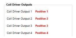
This will indicate how many drivers are allocated to coils and their connection pinout on your product. It may change according to Coil Driver Trigger Combination setting. This will allow the installer to do a printout of the drivers after setting up his unit.
