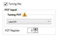
This feature controls the way the engine handles the Turbo or tuning of Fuel or Timing. It does not affect wiring but can be dangerous if it controls fuel or ignition timing.
