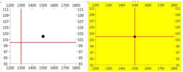
The focus window guides the tuner to the centre of the block so that his tuning is accurate. Otherwise he will tune the wrong values in the active block. He will need to fine adjust the Dyno RPM's and adjust the load with his foot till the window turns yellow.
