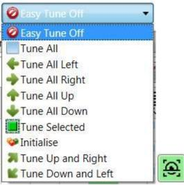
Easy tune and real time tracking are very useful tuning tools in this tuning pallet. It assists the tuner to tune where the load and RPM is without moving the tuning block with the arrows.
