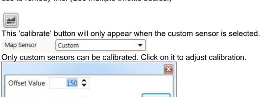
If you click calibration this block will appear. The offset value will change the MAP reading. Adjust it to read the same as the barometric pressure of your altitude above sea level. **Note**: Remember to take temperature into account.
