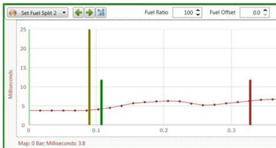
Now adjust the fuel to increase as the TPS is increased so that the flat spot is corrected. If you don't find a sweet spot between the TPS fuel and MAP crossover, then you may need to move the Vacuum Fuel Cut-off higher to 0.2 Bar. This will have a higher value on the Fuel economy cut and result in harsh control on that feature.
