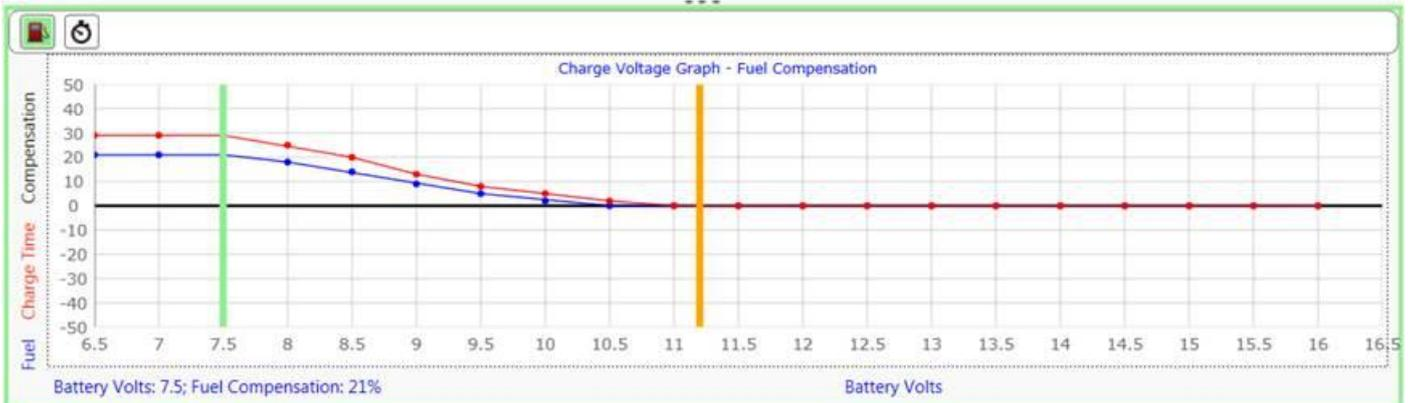
Make sure that fuel compensation is zero at operating voltage in the Charge Voltage Graph.
