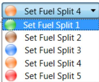
Set the 5 tune markers in even space over the load of the engine. The green marker could be at idling and the red high bar at about 90% load. Space the other ones evenly.
