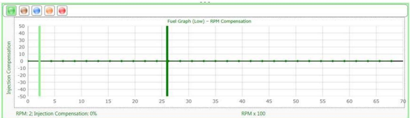
Zero all 5 graphs on the Fuel Graph – RPM Compensation.
