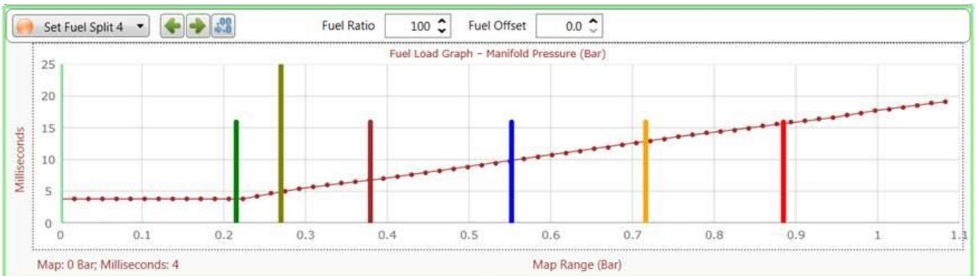
Your main fuel map should look something like this. This means engine idles at around 0.2 bar vacuum and requires 4 milliseconds of fuel to idle when hot. The slope will provide enough fuel to rev and ride the engine. If your injectors are larger than standard, then idle fuel would be lower and the slope less aggressive. Note: Fuel Ratio is set at 100% and Fuel Offset is as 0%.
