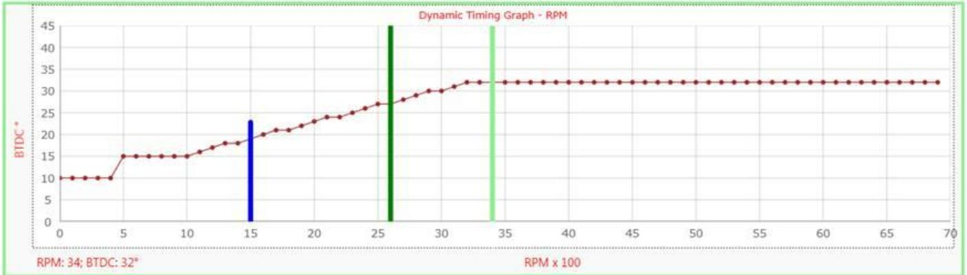
This is a basic dynamic timing that should work for the average engine. Set a basic RPM timing map to start at 10° BTDC degrees and idle at 15 °BTDC degrees. Increase the timing from 1000RPM to 3200RPM up to 32° BTDC. Keep it flat till maximum timing. If you have a special engine with high compression, then lower the maximum timing to 28 degrees.
