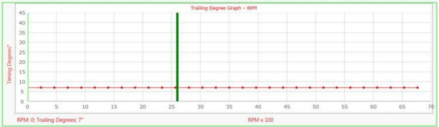
If you have a Rotary engine also set the trailing degrees at a base timing of 7 degrees.
