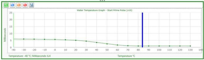
The Spitronics ECU's have a manual prime function where you can press the accelerator pedal before starting to inject fuel in the system. This fuel is measured at 50% of the start prime pulse setting. It is injected each time the throttle is pressed more than 25 % opening.
