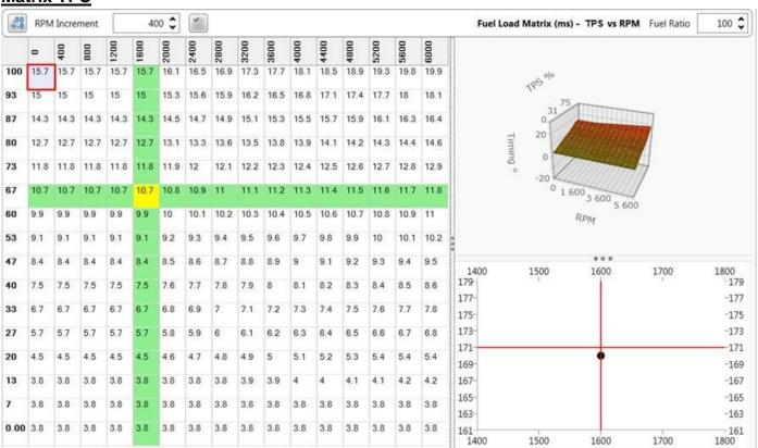
This is for normal aspirated engines with poor vacuum signal or throttle bodies and allows for easy dyno tuning. Note: It is recommended to add the altitude sensor to compensate for altitude pressure changes. TPS versus RPM does not compensate for pressure changes. Here the TPS sensor versus RPM is used and the blocks are set in 0.1 milliseconds resolution.
