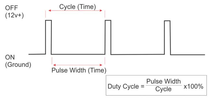
A fuel injector is continuously powered by battery positive. The ECU output switch to ground to turn the injector 'on'.
