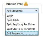
This setting will allow different methods of fuel injection. The firmware in the ECU will blank out the methods that are not adjustable. In some firmware a refresh will be forced to reshuffle GP outputs or cancel an illegal setting.
