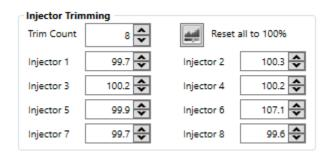
This feature allows the tuner to trim each injector individually for the ultimate performance. This is done by individual Lambda or EGT sensor on the exhaust runner to measure individual air fuel ratios. It is only selected Mercury2 firmware that has this feature.
