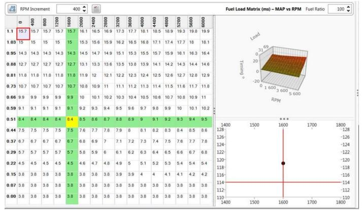
This is for standard engines with a good vacuum signal and allows for easy dyno tuning. Here the MAP sensor versus RPM is used and the blocks are set in 0.1 milliseconds resolution.
