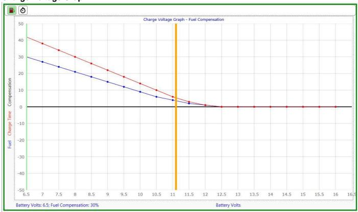
The blue graph adds a certain percentage to the injector time and the red graph adds a certain percentage to the charge time. This is not an easy one to tune but it is recommended to lower the values and see if the result is worse or does not make a difference in starting. Always go for the lowest values. You may also decrease the values with higher battery charge. This may help protecting the coil drivers. These graphs are interpolated.
