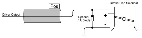
**Note:** The connection to the ECU changes with the GP Output Priority selection, View the Pin Layout spreadsheet for the specific firmware to see which output is selected. Then make sure on how to connect between the 2 options above. It could be connected on a negative or positive driver. Also make sure from the specifications for the driver that it can handle the current rating for your specific cam solenoids.
