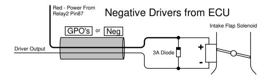
**Note:** Make sure the stripe of the Diode is connected on the positive side.
