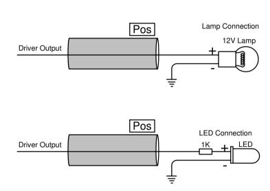
**Note:** The connection to the ECU changes with the GP Output Priority selection, View the Pin Layout spreadsheet for the specific firmware to see which output is selected. Then make sure on how to connect between the 2 options above. It could be connected on a negative or positive driver. Also make sure from the specifications for the driver that it can handle the current rating for your specific cam solenoids.
