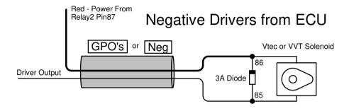
**Note:** Make sure the stripe of the Diode is connected on the positive side.
