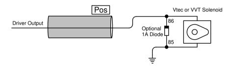
**Note:** The connection to the ECU changes with the GP Output Priority selection, View the Pin Layout spreadsheet for the specific firmware to see which output is selected. Then make sure on how to connect between the 2 options above. It could be connected on a negative or positive driver. Also make sure from the specifications for the driver that it can handle the current rating for your specific cam solenoids.
