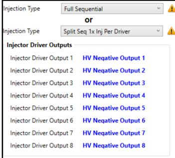
**Note!**: The software shows 8 drivers but only 4 drivers may be installed. Then connect 2 Injectors per ECU Driver
