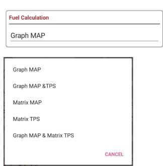
This block will allow the tuner to choose different options to set up timing for this engine. Each of these methods will be discussed in detail under the tuning chapter further in the manual. You can see the *Tuning* section for detailed description on the tuning side.
