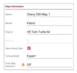
The Map information screen, **Name Model** and **Engine**, contains info for the ECU application for a specific vehicle. This helps the tuner to recognize previous work and tuning data. It is saved in the ECU and also in PC maps. It does not affect any tuning on the engine.
