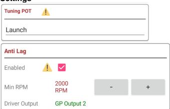
Enable the feature and set the minimum RPM setting. This RPM setting is the limit which will disable the function. If the engine revs fall below this value normal fuel economy cut will resume. During racing the driver will gear down keeping the engine revs high.
