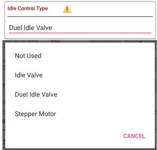
The *Type Selection* can select between the two-wire spring-loaded *Idle Valve*, the three-wire spring or non-spring loaded *Dual idle valve*, the Bipolar *Stepper motor* or common supply *Stepper motor*. Stepper motors do not use the Low Limit and High Limit settings as they keep their position when there is no signal present. If there is no idle control, select '*Not' used* to free up valuable processor time and general purpose outputs.
