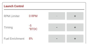
The launch settings *Timing* and *Fuel Enrichment* are also used for the Anti-lag feature. If it is activated, the timing will be retarded to the launch timing and the fuel will be enriched to improve burn pressure in the exhaust to spin the turbo.
