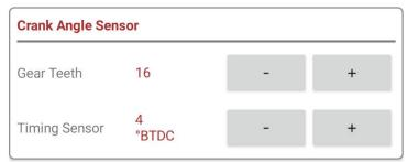
This block is used to indicate to the ECU where the exact TDC point is on the crank. It works differently for the different style of crank angle sensors. These settings will allow the ECU to synchronize software timing with the actual spark timing on the engine.
