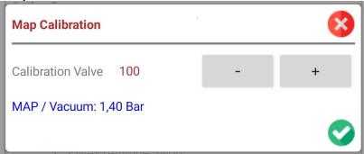
The offset value will change the MAP reading. Adjust it to read the same as the barometric pressure of your altitude above sea level. **Note**: Remember to take temperature into account.
