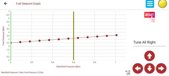
This graph will adjust the Fuel Pressure versus Load.
