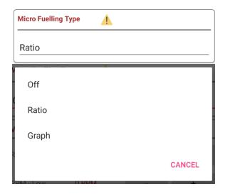
Select the type of injection method to use for dual injectors.
