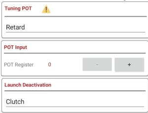
Set the RPM limit on zero. Set the launch control timing on 5 to 15 degrees depending on the feel of the shift in the transmission. Launch deactivation must be on Clutch. Fuel enrichment is not used here.
