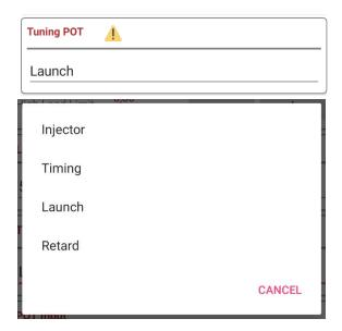
**NB!** This is a Critical setting that alters wiring connections. Do not change it on a running vehicle. It could damage drivers or components on the engine.
