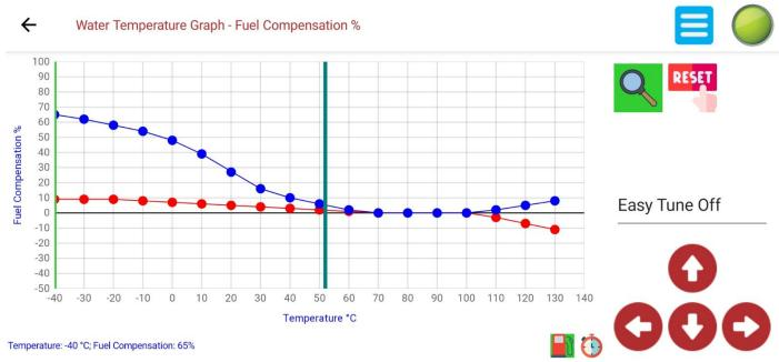
This graph will adjust Injection Time compensation versus Engine Temperature. Y-Axis Blue = Injection Time Compensation in percentage from -50% to 100%. Y-Axis Red = Ignition Timing Compensation in ° BTDC from -50° to 100° X-Axis = Temperature value of engine from -40°C to 140 C.
