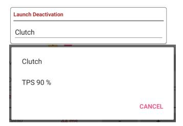
There are 2 methods to deactivate the Launch feature. *Clutch* is with hardwire switches and *TPS* **90%** is for a semi-automatic method.
