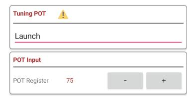
Now set the *POT register* to your engines maximum RPM plus 500rpm. If engine can rev to 7000RPM then select 7500RPM. The reason is that this POT is also used to deactivate the launch control by adjusting launch RPM higher than the engine can achieve. Simply turn the POT fully clockwise.
