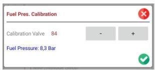
If you have an accurate fuel pressure gauge or a different fuel pressure sensor you may calibrate it with this value. It is a percentage correction which allows for range calibration only. That means calibration is accurate at the working pressure. The sensors supplied are calibrated according to the manufacturer signal specs. See the *Fuel Pressure Sensor Settings* page for other adjustments.
