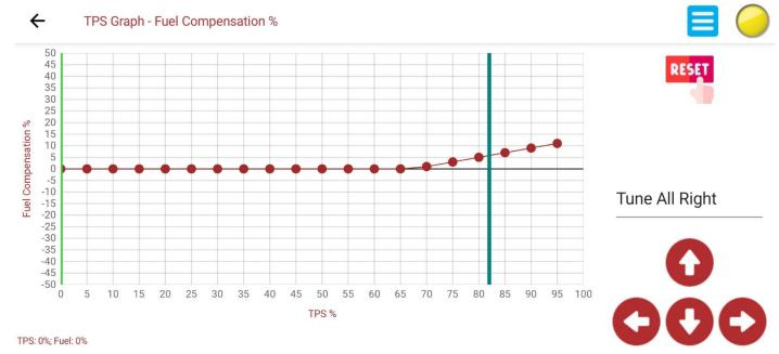
This graph will adjust Injection Time compensation versus TPS position. Y-Axis = Injection Time Compensation in percentage from -50% to 50%. X-Axis = TPS value of engine from 0 to 100%.
