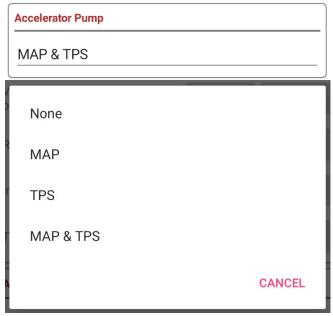
The accelerator pump setting is used to richen the fuel mixture when accelerating to avoid flat spots or bog. Here you can select not to use it, use either the TPS or MAP or both signals. Below is the selections to setup each pump for TPS and MAP.
