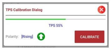
The TPS value must increase with throttle depression. If it is decreasing, click on *Polarity* to select *Negative*. This feature is normally used where the original ECU is still connected and wiring cannot be altered. In this case you connect only the ECU TPS signal wire to the OEM signal wire. Do not connect the ground or 5-volt signal wires but isolate them to prevent shorts. Now click the *Calibrate* button. The current TPS value will be written into the two blocks *Min* and *Max*.
