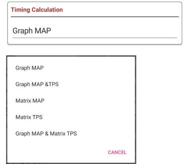
This block will allow the tuner to choose different options to set up timing for this engine. Each of these methods will be discussed in detail the Hyperspace Timing settings Manual.
