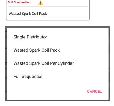
This block indicates the type of coil combinations that can be used with this firmware. Firmware will block out the ones that is not allowed. On some if you select a wrong combination the software will refresh and cancel your selection. If you have an intermediate or lower hardware class ECU, it will also hide the multi coil settings. Most COP coil per cylinder engines are fired in wasted spark configuration and each coil will have its own driver. (See the wiring diagrams for connections.)
