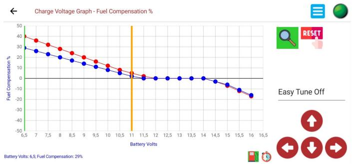
This graph will adjust Injection Time compensation versus Battery Voltage. Y-Axis Blue = Injection Time Compensation in percentage from -50% to 50%. Y-Axis Red = Coil Charge time Compensation in percentage from -50% to 50% X-Axis = Battery Voltage value from 6.5V to 16.5V.
