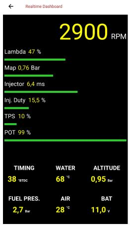
This block displays all the analogue sensor values as they change in the ECU. Below is a description of the meaning of each signal.
