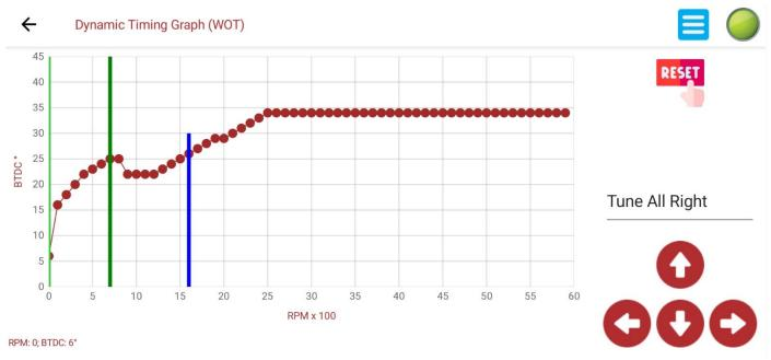
This graph will adjust Ignition Timing versus Engine RPM.
