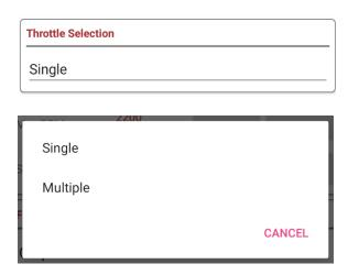
This setting is developed to use a MAP signal on multiple throttle body engines. The problem with them is there is no intake plenum where the vacuum could be measured. The vacuum signal only makes a spike when the valve opens. This spike is also there only once in two RPM's. This makes it important to read the signal on crank degrees when the vacuum signal is present. This setting is only available for gear type triggers as low as 12 teeth.
