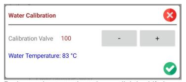
Reduce or increase the value to slightly shift the reading value. Do this at the critical temperature for instance where the fan must come on or off. If the error is too large you may need to replace it or get the correct sensor. These sensors are measured at 25°C with an ohm meter to see which type it is. If you have the wrong type you may need to change the sensor to a 2K sensor. Save to
