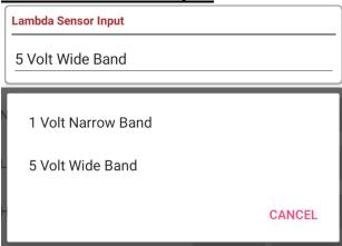
This input is used to select between a narrow band 1 volt signal and a wideband 5 volt signal. A wideband signal is linear and can cover a wider range of A/F measurements. It can be used for idling and high load readings. Notice that the rich and lean % change between the 2 sensors. Narrowband is inverted and wideband is linear.
