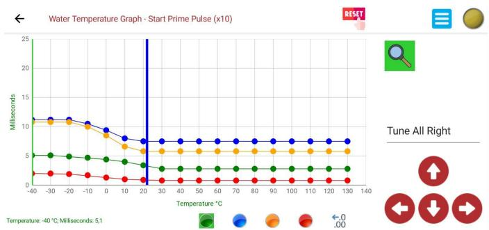
This graph will adjust Prime Pulse, Start Enrichment, Accelerator Pump Map and TPS signals versus Engine Temperature. It is only visible in Expert Tuning Mode.
