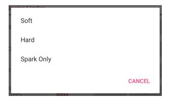
You may select the type of engine cut which is the same as the normal rev limiter settings. Soft will cut only fuel, Hard will cut fuel and spark and Spark Only will cut spark.
