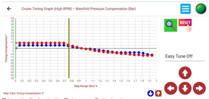
This graph will adjust Ignition Timing versus Engine Load.
