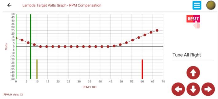
This graph will adjust Lambda Target Volts compensation versus Engine RPM. Y-Axis = Lambda Target Volts compensation in percentage from -50% to 50%. X-Axis = RPM value of engine from 0 RPM to 15000 RPM
