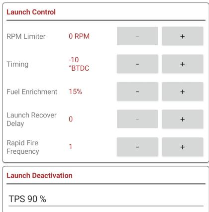
Set the desired *RPM limit* to 0. This will indicate to the ECU that it must use the POT value to calculate a RPM limit value. Set the desired *Timing* and *Fuel Enrichment*.
