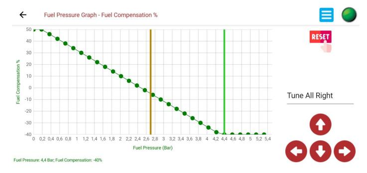
This graph will adjust Injection Time compensation versus Fuel Pressure. Y-Axis = Injection Time Compensation in percentage from -40% to 50%. X-Axis = Fuel Pressure value from 0Bar to 7Bar.
