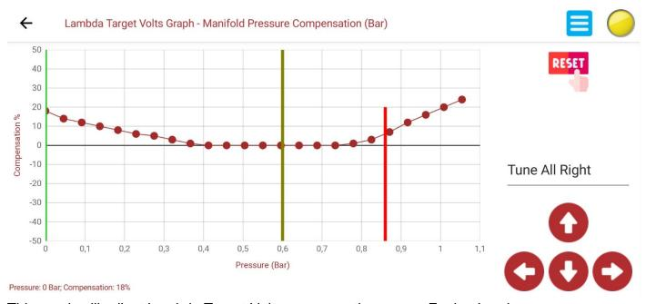
This graph will adjust Lambda Target Volts compensation versus Engine Load. Y-Axis = Lambda Target Volts Compensation in percentage from -50% to 50%. X-Axis = Load value of engine. Can be MAP Sensor or TPS sensor
