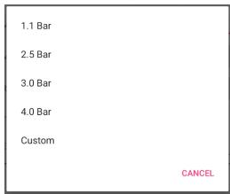
Spitronics have a selection of 4 Map Sensors to choose from. 1.1 Bar, 2.5 Bar, 3.0 Bar, 4.0 Bar and a Custom sensor option. Select the one that is supplied with the ECU. The most popular one is 2.5 Bar.
