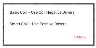
This block selects the coil type connected to the ECU. There are Basic Coils that requires an HV Coil driver and then there are Smart Coils that has built in drivers.
