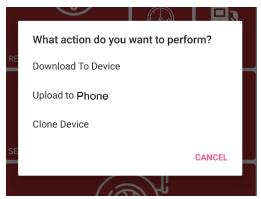
Download to Device means the map will be loaded in the ECU but the Critical Settings will not be changed.
