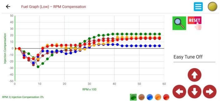
This graph will adjust Injection Time versus Engine RPM on 5 graphs. Each graph operate in a certain load section determined by the selection bars in the Fuel Load graph above.
