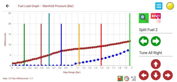
This graph will adjust Injection Time versus Engine Load.
